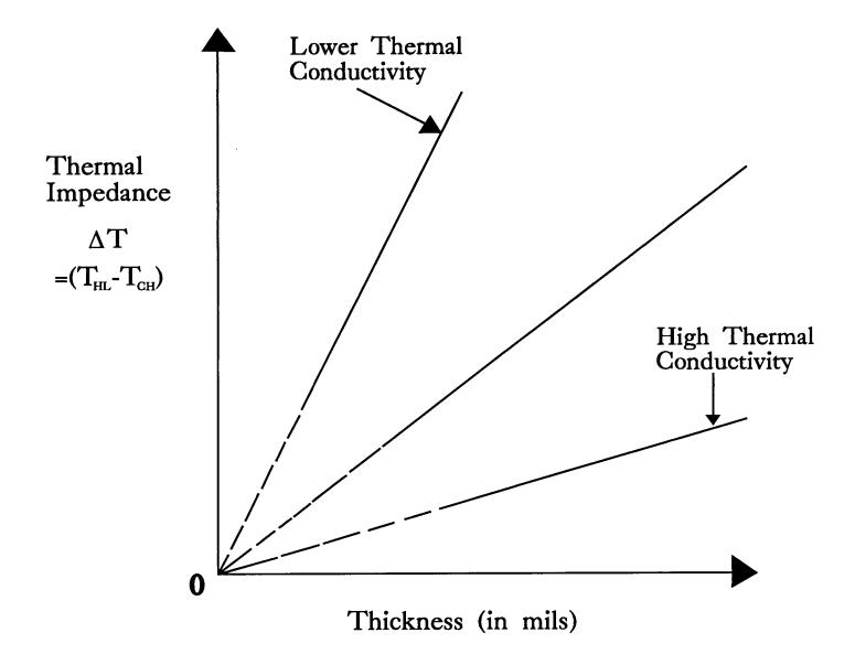
Figure #2: Theoretical Dependence of Junction Temperature of Bond-line Thickness and Thermal Conductivity of Adhesive
