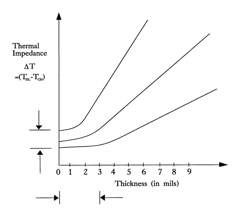
Figure #3: Thermal Impedance Effect of Interfaces in an Adhesive Assembled Electronic Device
