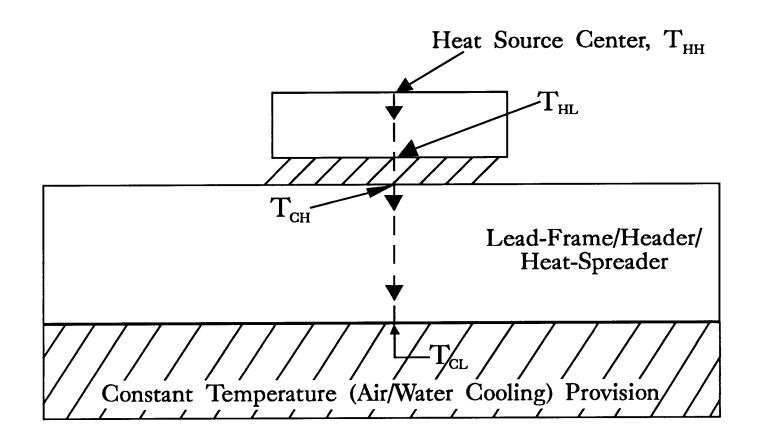
Figure #1: Schematic of an Adhesive Assembled Device
