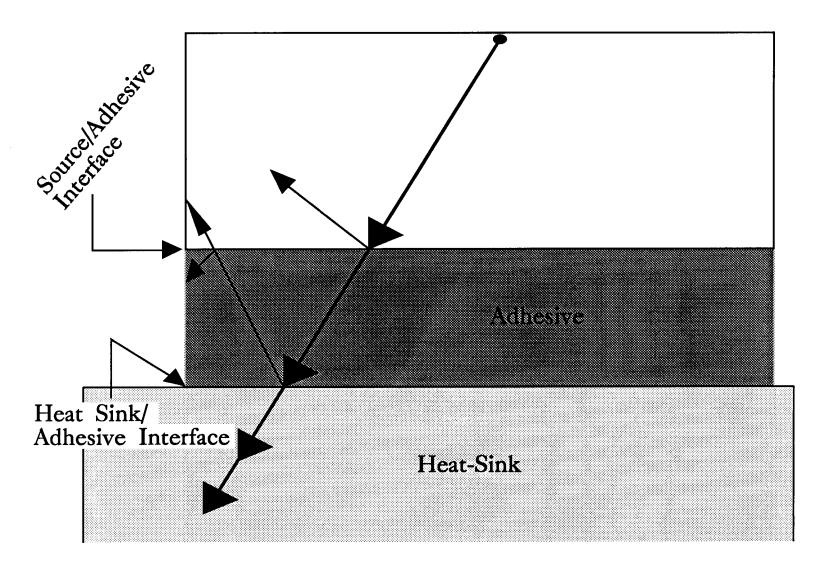
Figure #4: Schematic of Phonon Scattering at the Interfaces of an Assembled Electronic Device
