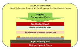
WPA-TS-320, WPA-TS-300 and WPA-TL-330 Support Heat-Sliding Separation-Debonding at 250-300°C with Shear Forces
