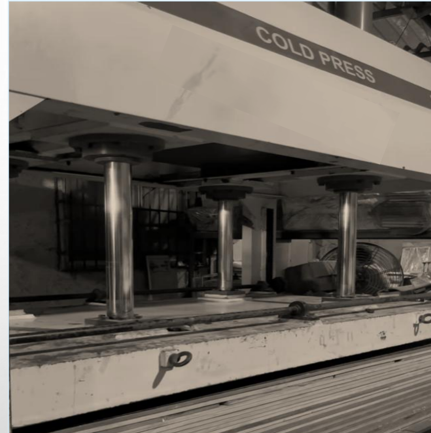
(3) Laminate Bonding with Cold Press or Calender Rolling Pressure for Flatness
