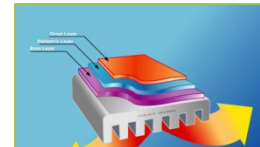
Insulated Metal Thermal Substrate for Large Area LED
