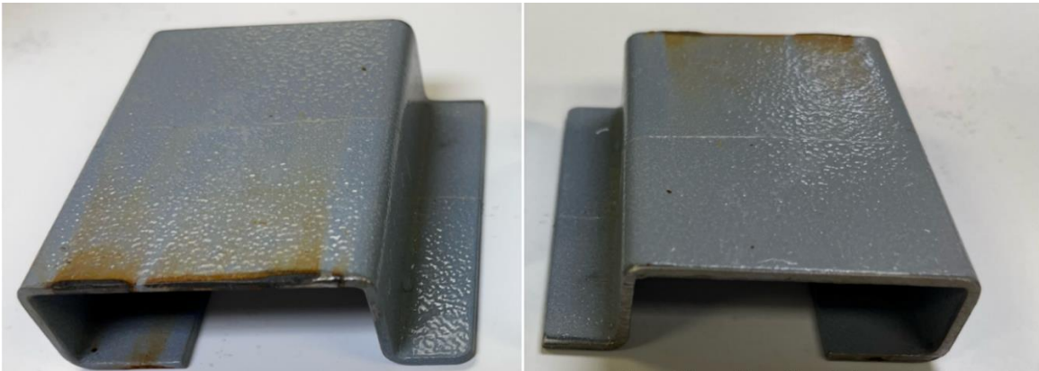
Figure 11: FBE coated edges corrode quickly upon exposure to 5% salt water at accelerated temperature of 60°C after 50 hrs. The corrosion quickly propagated outward to other areas. The new PVDF Corrosion Protection Coating is used to coat on the side that was cut with exposed bare steel. No sign of corrosion is seen under the same salt water condition. The new PVDF Corrosion Protection Coating is transparent having a thickness of approximately 30 \mu m, applied by brush and ambient dried.
