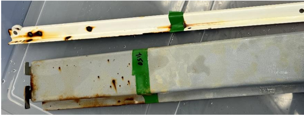
Figure 12: Steel bars coated with epoxy coatings, are partially coated with field applicable 100% PVDF top coat (~50µm thickness). The portion protected by epoxy coatings only when exposed to salt-water (water with dissolved corrosive ions) suffered extensive corrosion in 65 days under the accelerated conditions of 60°C-5% saline solution. By comparison, epoxy coated steel when top coated with field applicable PVDF coating showed no sign of corrosion. The accelerated conditions are roughly equivalent to 2-3 years of ambient temperature seawater submersion condition.
