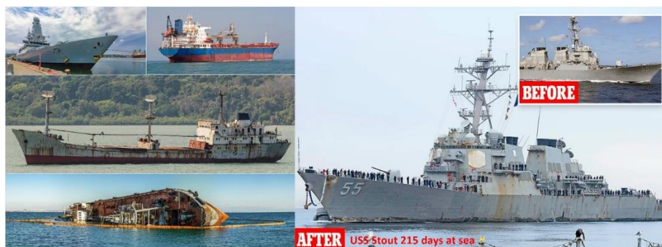
Figure 1: Marine and naval assets show significant corrosion both above and below the sea waterline after just a few hundred days at sea.
