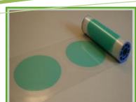
Lamination of wafer onto dicing die-attach film (DDAF)
