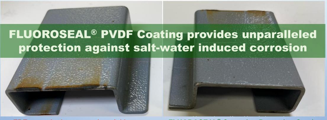
FBE coated edges corrode quickly upon exposure to 5% salt water. The corrosion quickly propagated outward to other areas.
