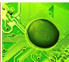
Glop-Top for Chip-On-Board Extreme Moisture and Stress Management
