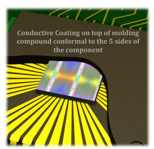
Component package conductive coating must attached to the molding compound:
