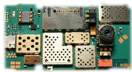
Individual component package with metal lid shielding is cost effective and technically viable for 3G and early 4G devices
