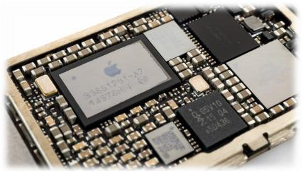
Component package conformal conductive shielding becomes a necessity for late 4G devices
