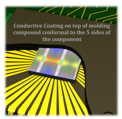
Component package conductive coating must attached to the molding compound:
