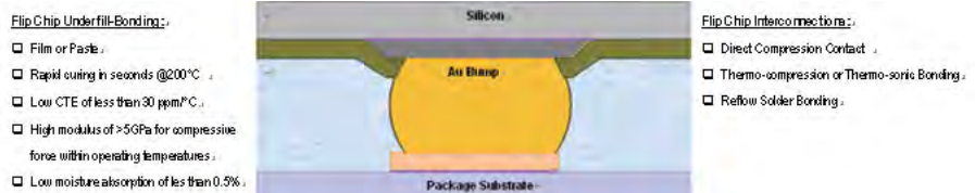
Figure 5. Flip-chip interconnection with direct mechanical contacts between precious metal bumps and preservations on chip and package substrate respectively
