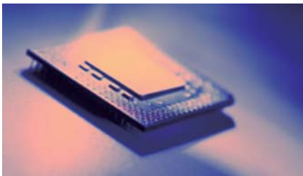
Figure 1. CPU is one of the great successes of flip-chip application
