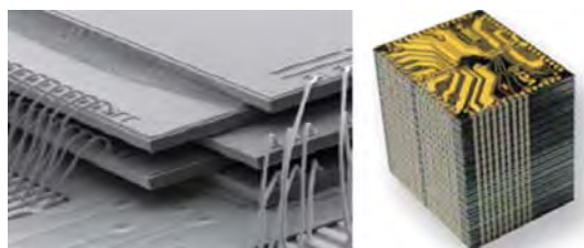
Figure 2. Stack-chip packages can be interconnected with wire bonding or special design inter-chip interconnection bridges
